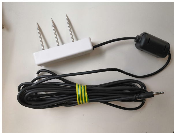
Figure 2.4: Teros 11 VWC capacitive sensor
