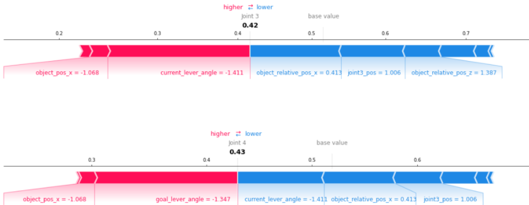
Figure 4.7: Robotic Manipulator: LIME Local explanations Joints 3 and 4
