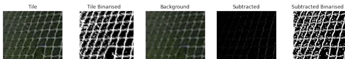
(a) Opening with a kernel size 25% The Elbow includes the Net Structure in the Background, which can break true mesh connections in the binary image and cause false positive irregularity detection.
