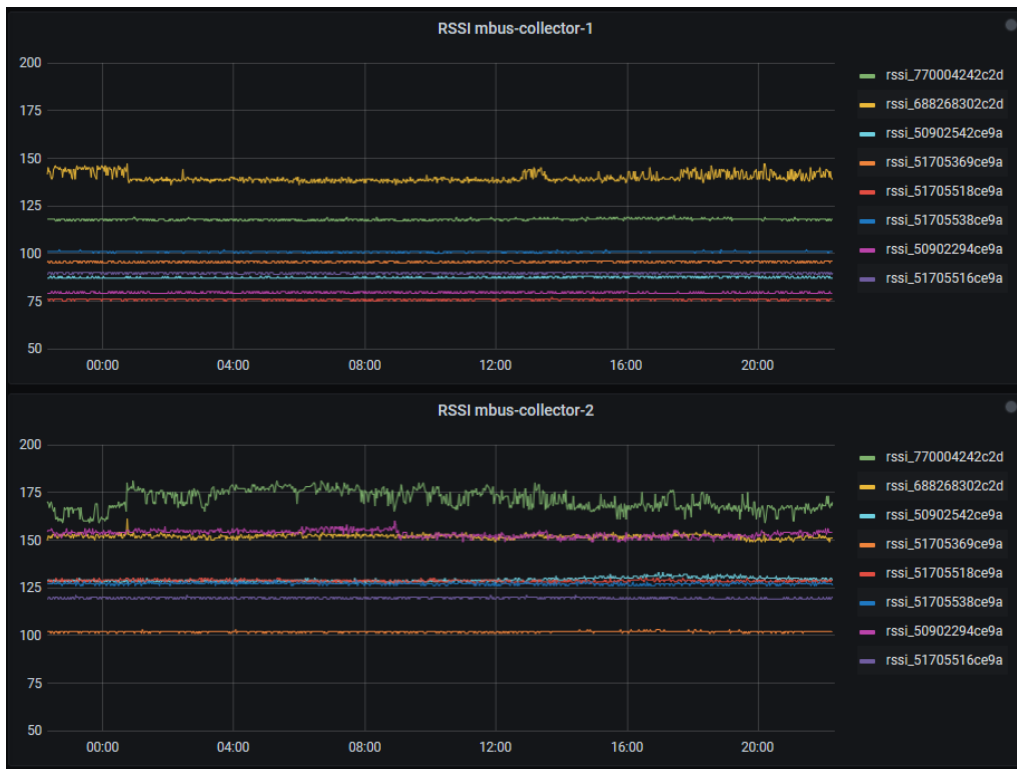
Figure 6.9: Grafana panel showing RSSI measurements from all meters for both collectors.
