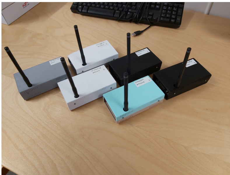
Figure 5.1: The simulated meters used in the project. 3d-printed boxes were made to protect the circuit while being placed at different locations to broadcast wM-Bus packets. The sides were open so that they could be easily turned on.
