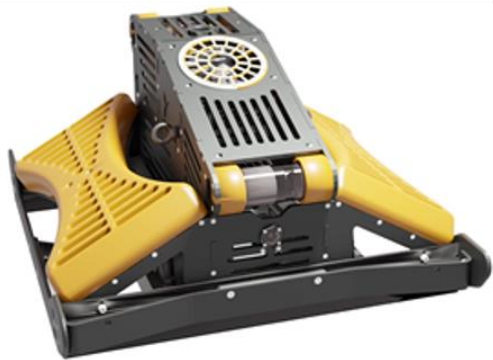
Figure 1: a) Remora biofouling prevention and net cleaning robot developed by Mithal AS, b) Simulation of the vehicle with two static regions of avoidance. The algorithm adapts the path, but not completely away from the regions of avoidance. The resulting path appears to be feasible.
