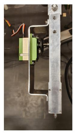
Figure 30: Servo pos "1"(Duty cycle 820000ns)
