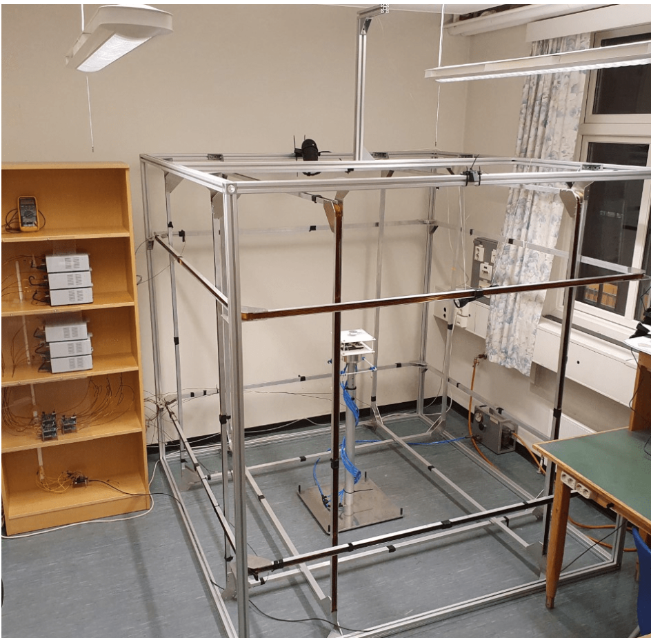
Figure 5.7: Image of the completed ADCS testbed.
