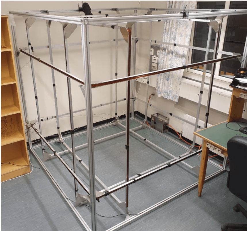
Figure 5.1: The completed Helmholtz cage.
