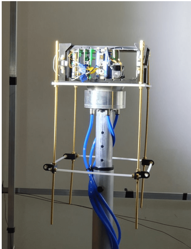
Figure 5.22: Orbit NTNU 2U satellite on test stand while being tested using sun simulator.
