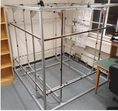
Fig. 2. Image of the completed Helmholtz cage.
