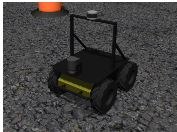
(b) Gazebo visualization of the Husky UGV, with 2D and 3D LiDARs.
