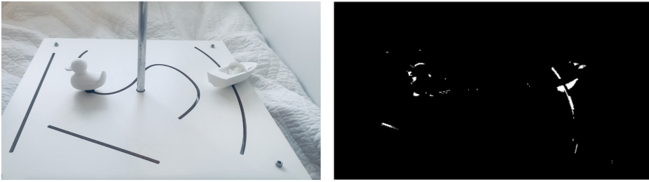
Figure 4.5: DMD results on foreground object with same pixel intensity as background object. The original frame frame is displayed to the left and the filtered foreground is displayed to the right.
