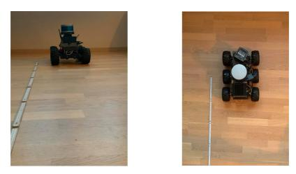
Figure 4.3: Calibration test of odometry.
