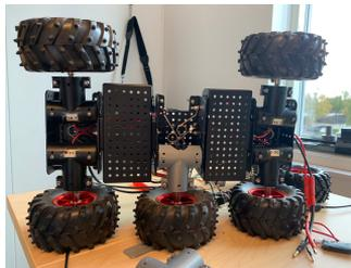
**Figure 3.3:** The bottom side of Phylax when one of the motors is removed due to reparations.
