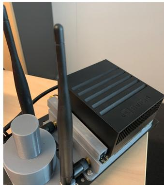
**Figure 3.6:** Nvidia Jetson AGX Xavier with antennas on the chassis. The gray part underneath the Xavier is the 3D-printed housing.
