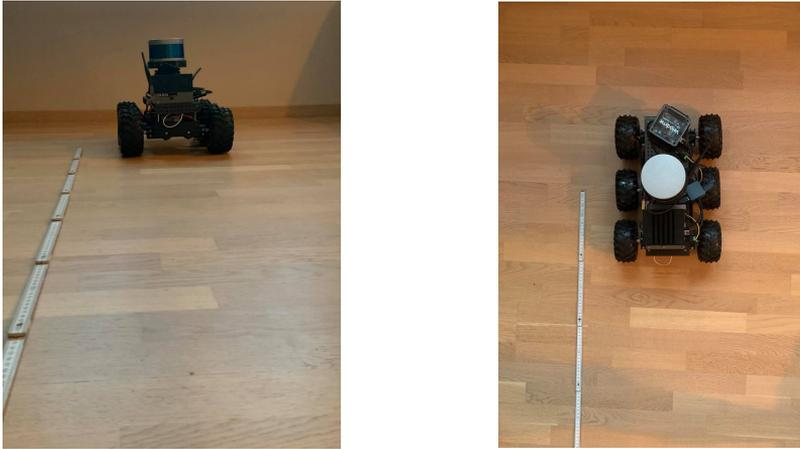
**Figure 4.3:** Calibration test of odometry.
