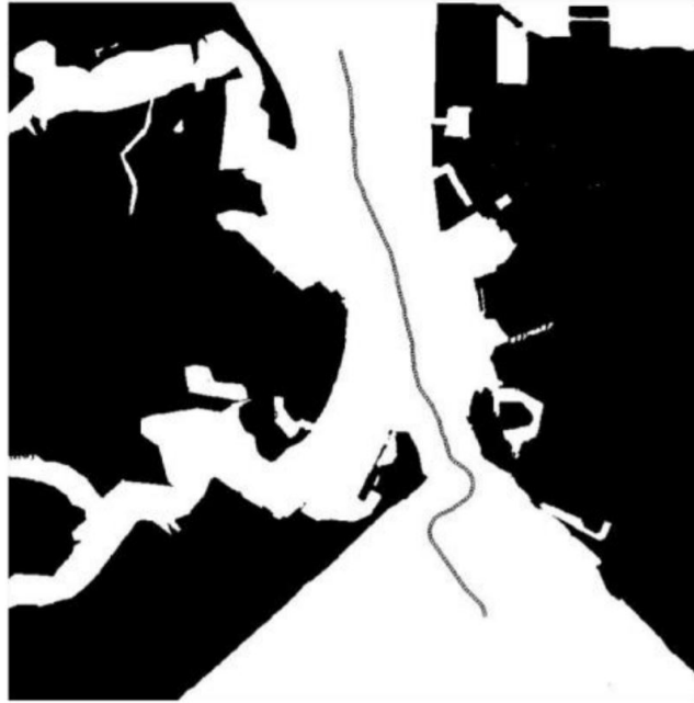
Figure 6: Potential field planning. Vessel starts at the bottom and moves up to the target at the top. Image: [12]
