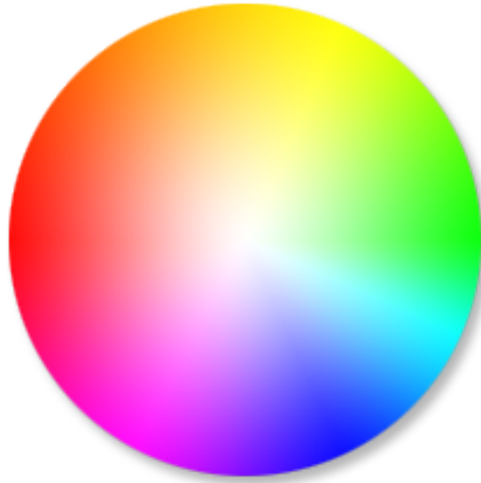
Figure 4.3: Color wheel used to represent pixel movement
