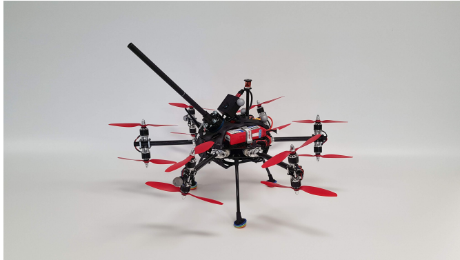
Figure 3.1: Ouzel the hardware necessary to perform contact inspection.
