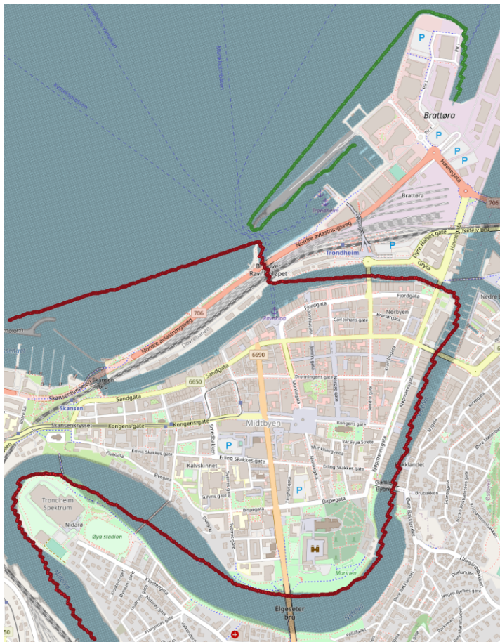
Figure 5.12: Paths created by PathPlanner on high-resolution grid.
