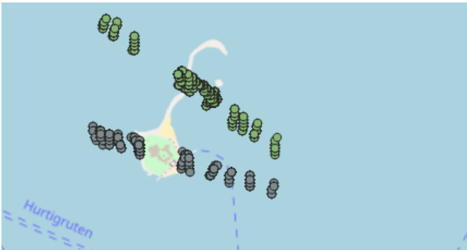
Figure 5.7: The results of running checkTransect on Munkholmen, Trondheim with contour vertices. Points show returned vertices with known DRVAL1 and DRVAL2 for each transect.
