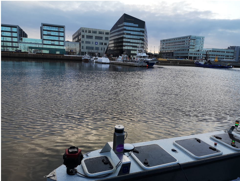
Figure 3.3: Old sensor setup where the LiDAR is mounted on top of a metal structure above the GNSS antenna, causing problems to find the heading of ReVolt.
