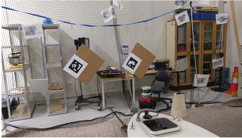
Figure 3.5: The calibration setup. The LiDAR and the camera may be seen at the bow of ReVolt.
