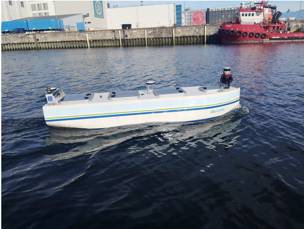
Figure 3.4: New sensor setup where the LiDAR is mounted on top the camera, and the GNSS antenna on a stand-alone structure in the middle of ReVolt.
