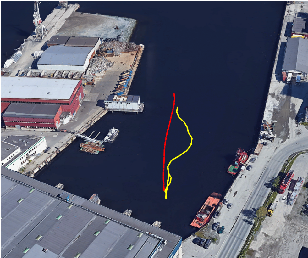
Figure 8.1: 3D photo of Dorabassenget where the experiments were conducted. The red and yellow line indicate the path of the obstacle and ReVolt respectively in the head-on scenario. The photo was obtained using Google Earth Pro and GNSS data from the experiment.
