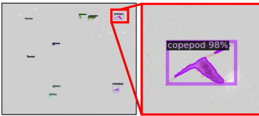
Fig. 3. From left to right: corrected background image and a zoomed cropped copepod of the framework end result. Overlay of inferred class, bounding box and segmentation mask from detectron2. Clearly, the copepod object is identified as one instance.
