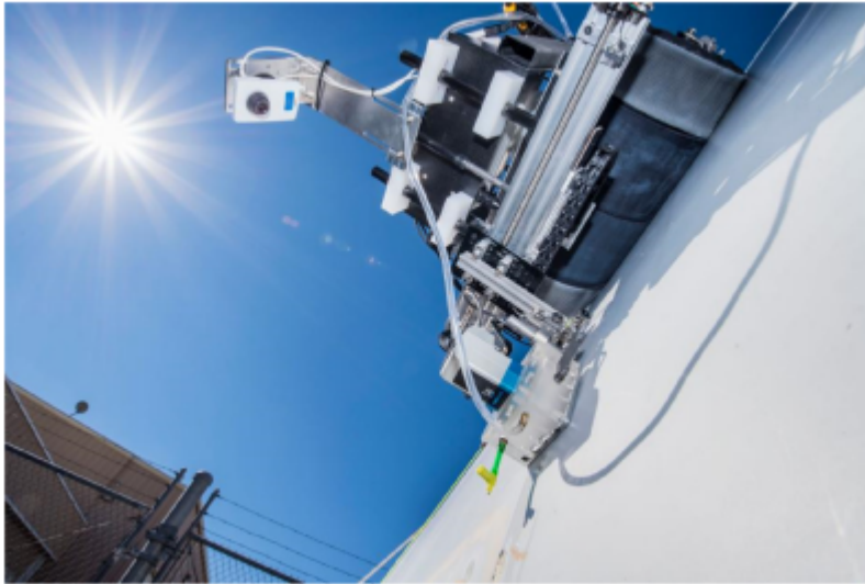
Figure 3.4: Sandia’s crawling robot with infrared cameras to look for hidden wind blade damage [44].
