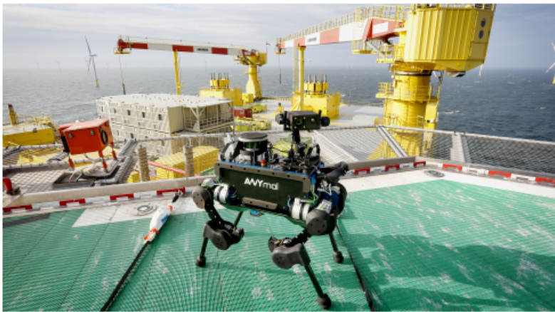
Figure 3.7: ANYmal deployed for autonomous inspection and surveillance on a wind energy HVDC converter platform in the North Sea [49].
