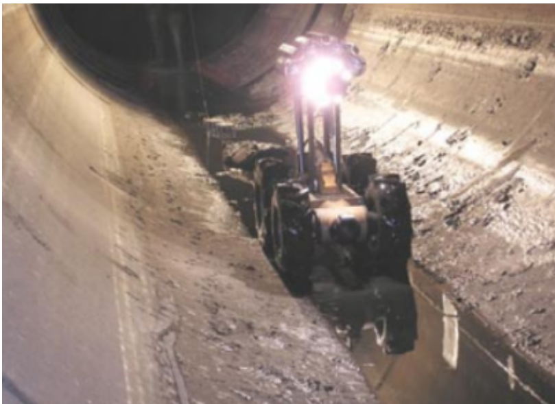
Figure 3.2: A standard crawler for sewage inspection according to [42].
