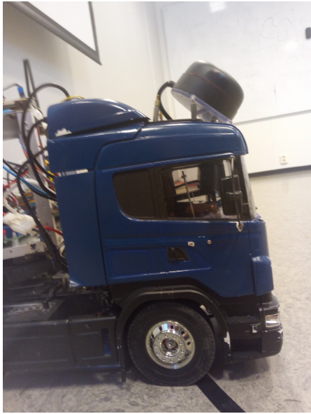
(a) Truck cabin with the Lidar mounted on top and the webcam mounted inside.
