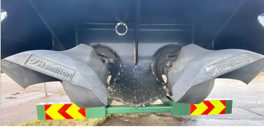
Figure 3.1: Odins two waterjets and deflectors seen at the stern of the vessel. Courtesy of FFI.
