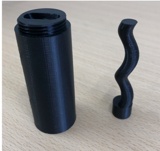
Figure 4.10: 3D-printed plastic version of stator and rotor.
