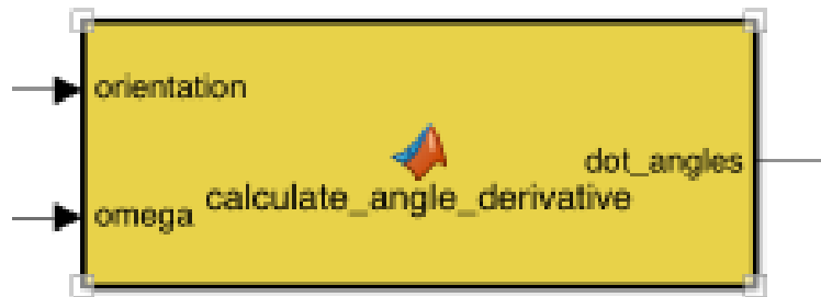
Figure B.2: The Matlab-function block used to calculate the angle derivatives \dot{\phi} , \dot{\theta} and \dot{\psi} .
