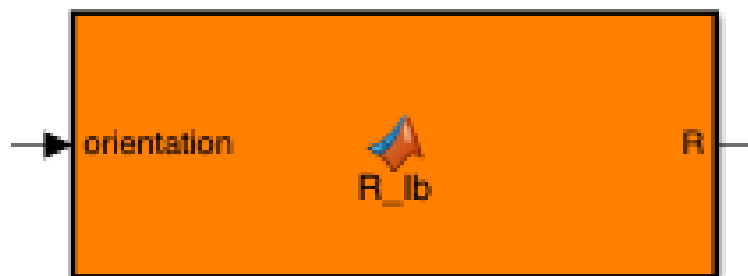
Figure B.5: Matlab function block used to rotate the ROP from \{b^c\} to \{I^c\} .
