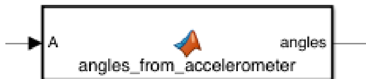
Figure B.1: The Matlab-function block used to calculate \theta and \psi using measurements from an accelerometer.
