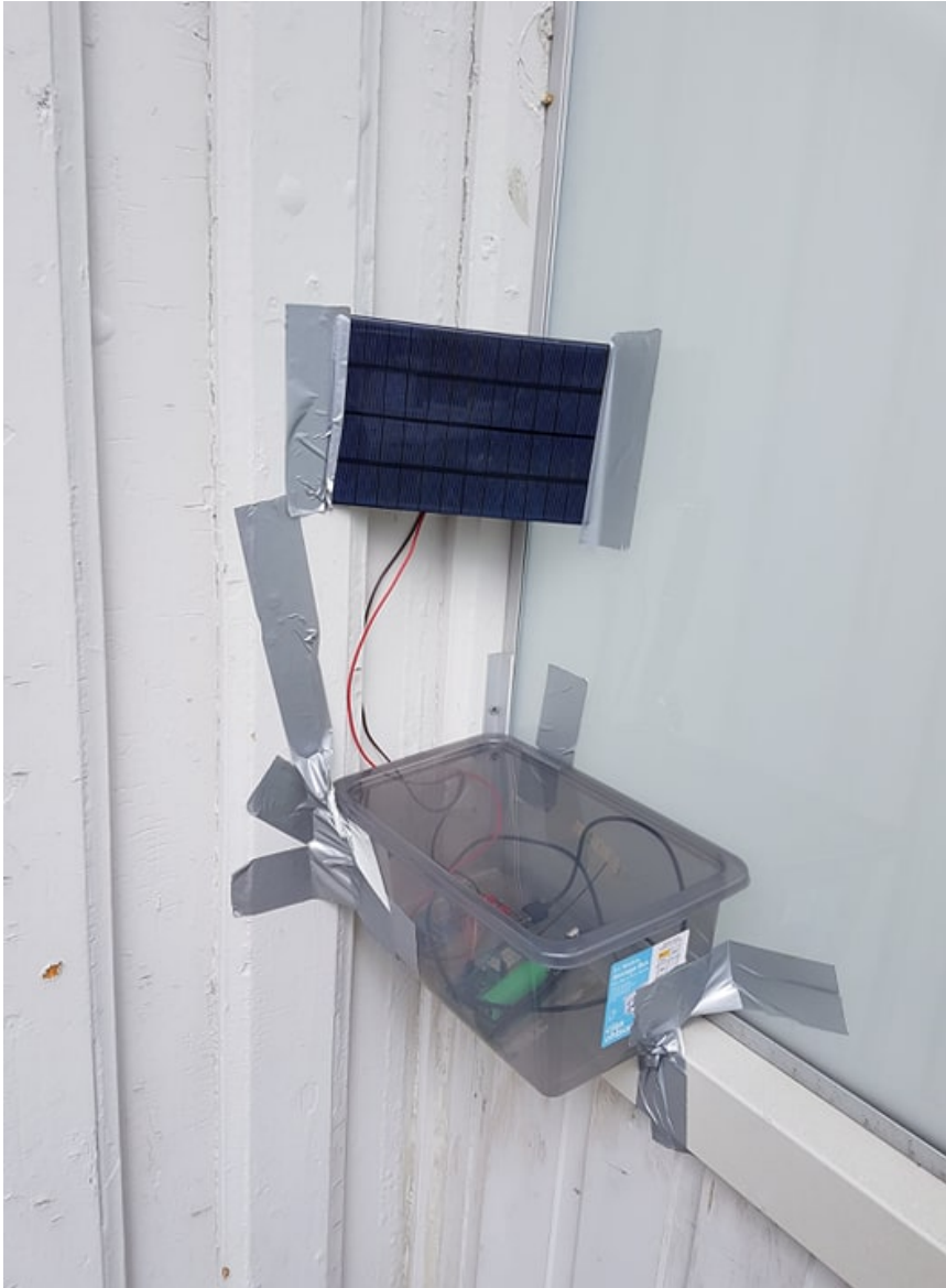
Figure 5.23: Deployed LoRa-node 3. Outside with no roof.
