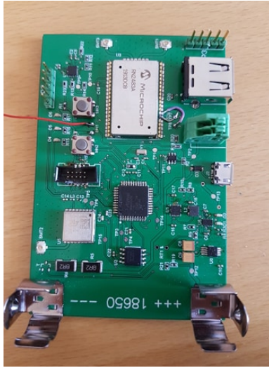
Figure 5.9: Assembled end-node without battery for original solution.
