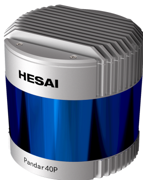
Figure A.4: The Hesai Pandar 40-channel LiDAR
