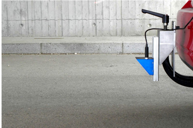
Figure A.2: The Pegasem GSS15 ground speed sensor.
