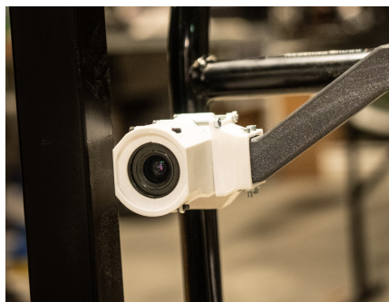
Figure A.3: The Basler acA1300-200uc USB 3.0 Camera
