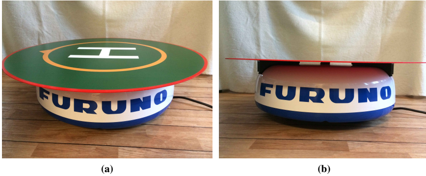
Figure 3.8: The finished landing platform attached to the radar.
