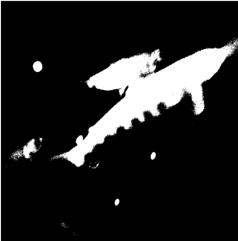
Figure 3.6: Resulting image when applying Otsu's method. This thresholding method has the worst performance. The reason behind this is the image histogram, which we see in figure 3.7. This algorithm wants to find a value between two peaks in the histogram, which makes the variances of the two classes minimal. As can see from the histogram, we only have one peak.
