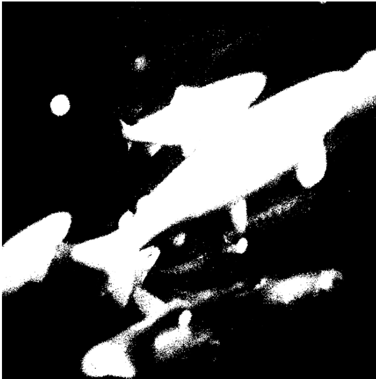
Figure 3.3: Illustration of the global thresholding method. In our case this method is very sensitive to the threshold value. The optimal threshold value is different for each image, making it unsuited for our application.
