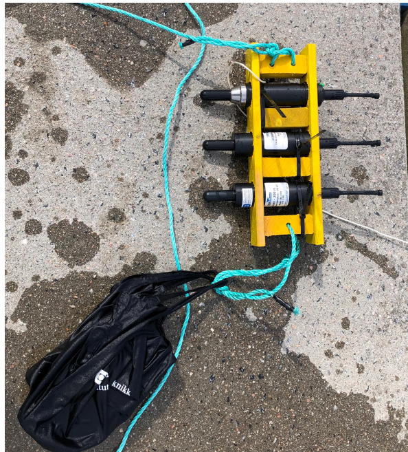
Figure 3.4: Hydrophones mounted to support frame with 0.1 m of separation. The tote bag contains a brick and works as an anchor weight holding the array still under water. The small white rope is used to point the array in the desired direction.
