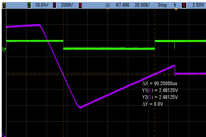
Figure 4.9: Oscilloscope trace illustrating the delay between the analog comparator falling edge, and the integrator changing direction. Channel 2 (in green) shows the immediate output from the analog comparator, and channel 3 (in purple) shows the integrator output. Channel 3 has an offset of 2.5 V
