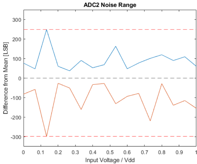
Figure 5.10: Plot of the noise for \Delta\Sigma ADC 2. The red dashed lines show the lowest deviation at -298.35 LSB, and the highest deviation at 248.65 LSB.
