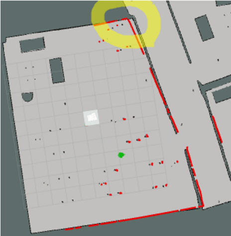
Figure 10.7: Incorrect values in Laser-Scan message header.
