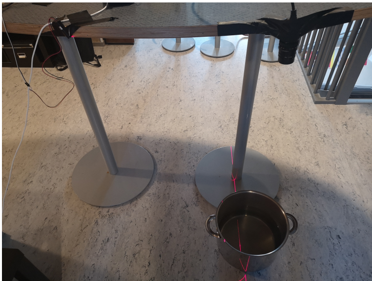
Figure 6.8: Example of the test-setup of laser depth measurement
