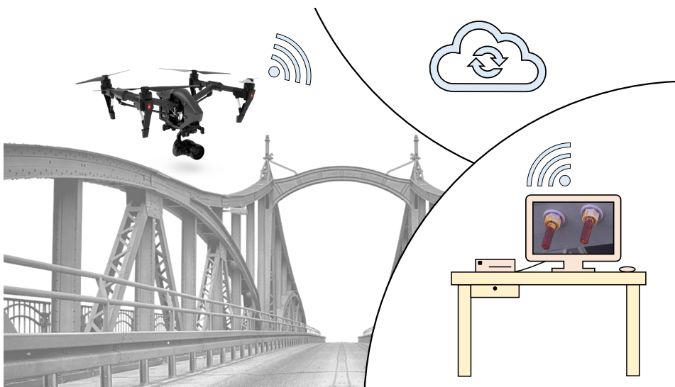
Figure 1.2: UAV inspecting a bridge. Images taken are wirelessly send, to a cloud service and a remote computer for further analysis. This removes the need for inspectors on-site, increasing efficiency and reducing costs and danger.
