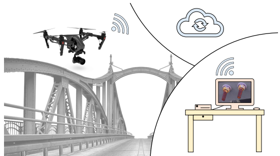
Fig. 1: Concept of a UAV inspecting a bridge. Images are sent to a cloud service/remote computer for further analysis.
