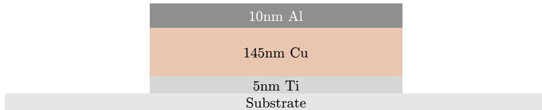
Figure 20: Illustration of a cross section the metal layers deposited using the lesker E-Beam evaporator. Not to scale.
