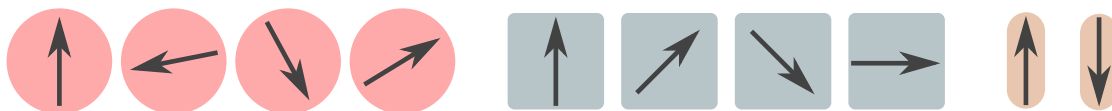
Figure 8: An illustration of a top-down view of several different shapes and magnetization directions for different shapes of nanomagnets.
