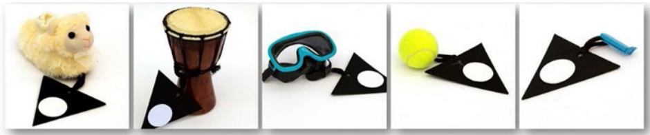
Figure 10. Familiar Common Arifacts with RFID-tag with virtual layer to change sound and graphics.
