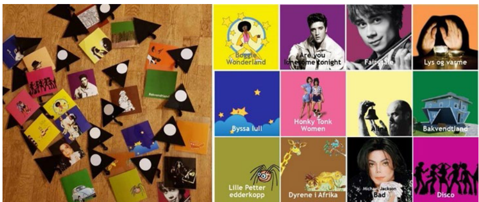
Figure 9. A few of the Scene-cards with RFID-tag on the floor. One control the music tune and colour graphics with the Scene-cards. By interacting, you can change the music and visuals dynamically.
