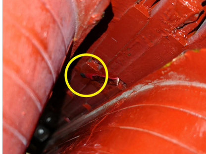
Fig. 9. The experimental test rig of a 100 kVA synchronous generator. The location of the hall-effect sensor installed on stator tooth
