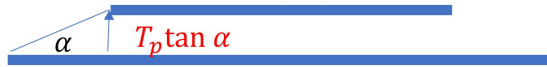
Figure A.2: Side view of the vertical tension component of two-torus model, connected by elastic bands. Courtesy to Trygve Kristiansen.
