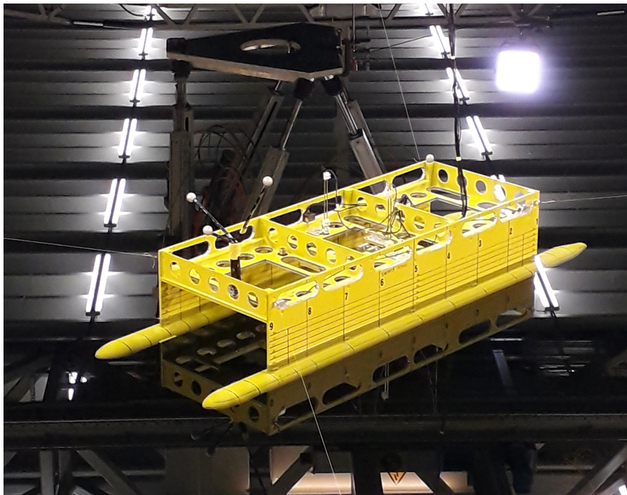
Figure 5.2: Model in the extended part of the main towing tank at Sintef Ocean in Trondheim, Norway. Here equipped without stabiliser fins and the ROV. The model is equipped with marker spheres to measure six DOF using Oqus and three accelerometers. The model is moored with four horizontal mooring lines.
