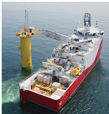
Figure 3.23: Siems ISV "Siem Moxie" operating on a foundation (Seaway7, n.d.)
