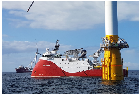
Figure 3.28: "Siem Moxie" during the commissioning of Hywind Scotland (Seaway7, 2017)
