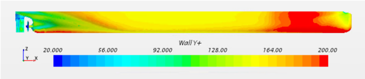
Figure 4.4: Y^+ value at different parts of the hull
