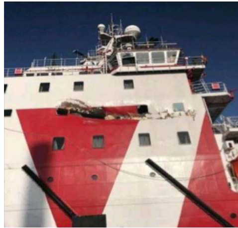
Figure 2.10: OSV damage after collision with OWT transition piece under construction. (Federal Bureau of Maritime Casualty Investigation, 2019)
