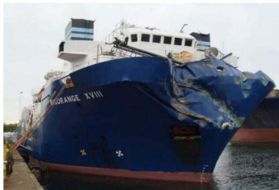
Figure 2.11: Big Orange bow damage after collision with water injection platform on the Ekofisk field. (Petroleumstilsynet, 2009)
