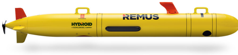
Figure 1.1: The REMUS 100 AUV
