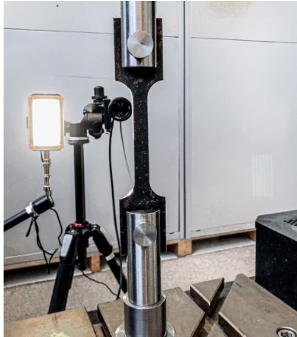
FIGURE 4.4: Setup for tensile tests with DIC.
