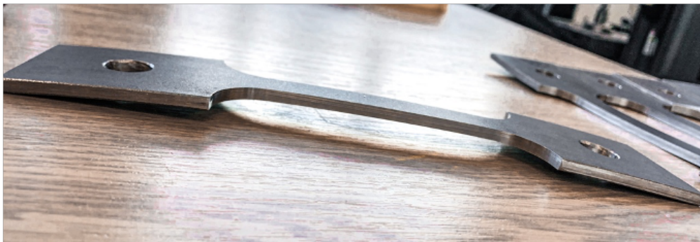
FIGURE 4.3: Visible curvature of coupon.
