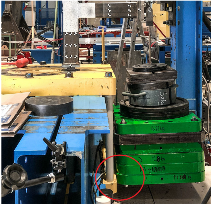
FIGURE 5.4: The green plate in the bottom was in contact with the yellow base plate for specimen C1B10M90.
