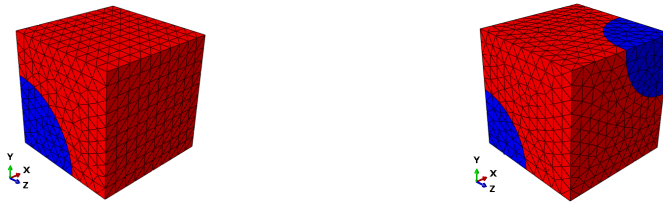
Figure 3.5: Docol 500DP: Illustration of the RVEs with spherical martensite. Martensite only in the centre to the left, while it is distributed both in the centre and the corners to the right. The blue and red parts represent the martensite and ferrite, respectively.
