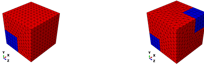
Figure 3.4: Docol 500DP: Illustration of the RVEs with cubical martensite. Martensite only in the centre to the left, while it is distributed both in the centre and the corners to the right. The blue and red parts represent the martensite and ferrite, respectively.
