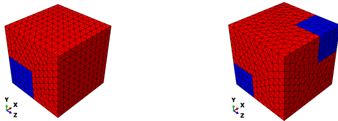
Figure A.1.1: Docol 500DP: Illustration of the RVEs with cubical martensite. Martensite only in the centre to the left, while it is distributed both in the centre and the corners to the right. The blue and red parts represent the martensite and ferrite, respectively.
