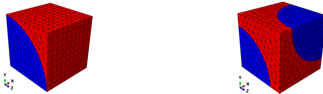
Figure 6.16: Docol 1000DP: The RVEs with spherical martensite where the volume fraction is 0.50. The blue parts are the martensite, and the red parts are the ferrite.
