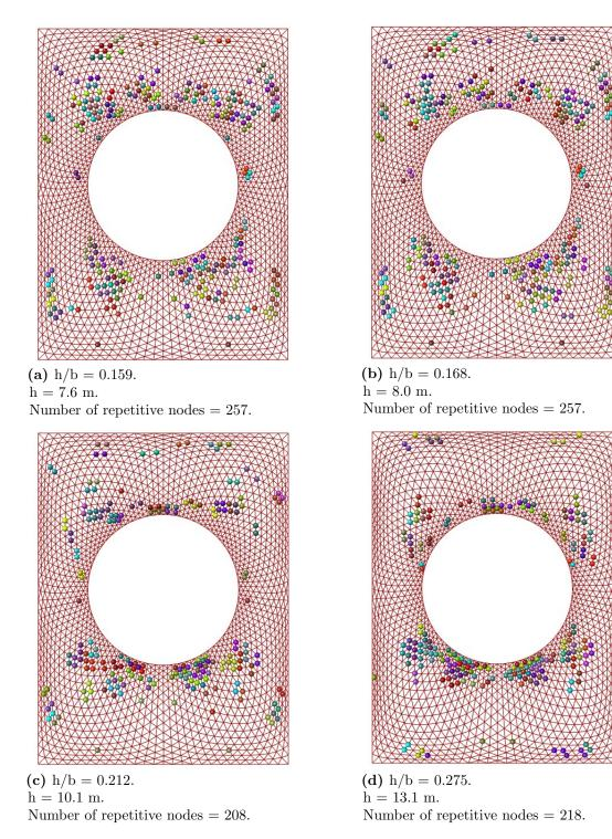
Figure 7.17: The distribution of the similar nodes for four different global shapes. +/-1 degree tolerance used.
