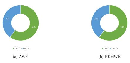
Figure H.2: CAPEX vs OPEX distribution for 3 TWh system.
