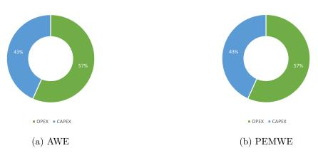
Figure H.1: CAPEX vs OPEX distribution for 1 TWh system.
