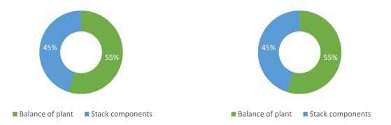
Figure 3.4: Cost breakdown of a 1 MW AWE Figure 3.5: Cost breakdown of a 1 MW [3]. PEMWE [3].
