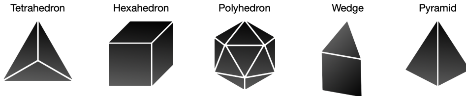
Figure 2.10: The most common types of three dimensional mesh elements.
