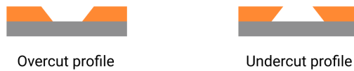
Figure 3.5: Schematic representation of the difference between an overcut and undercut resist profile for metal patterning.
