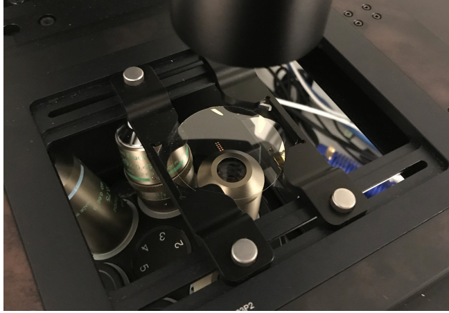
Figure 4.3: Experimental setup of the nanoplasmonic sensor displaying the microscope, objective, and a sample with 10 nanoplasmonic sensors.
