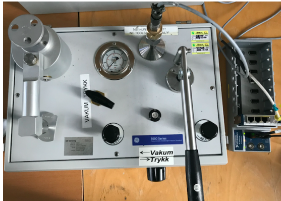
Figure 3.10: Experimental setup for the static calibration (low pressure range)
