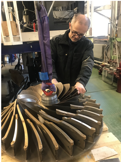
(a) Opland assembling the new blade
