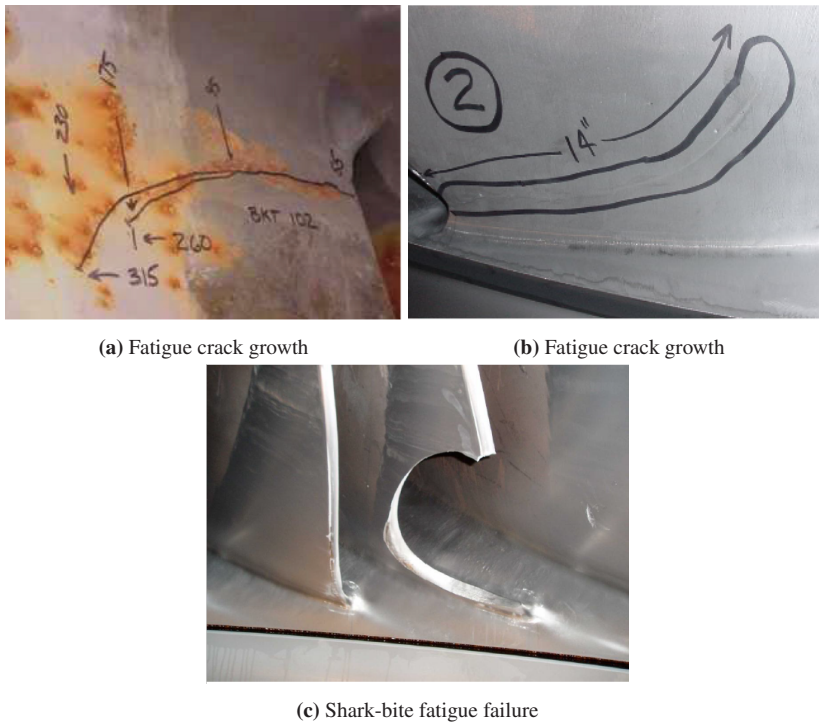
Figure 2.11: Three cases of fatigue damage occurring on the TE of a Francis runner blade reported by Liu et al. (a)[9], Cotou et al. (b) [10] and Fjærvoid (c) [11]
