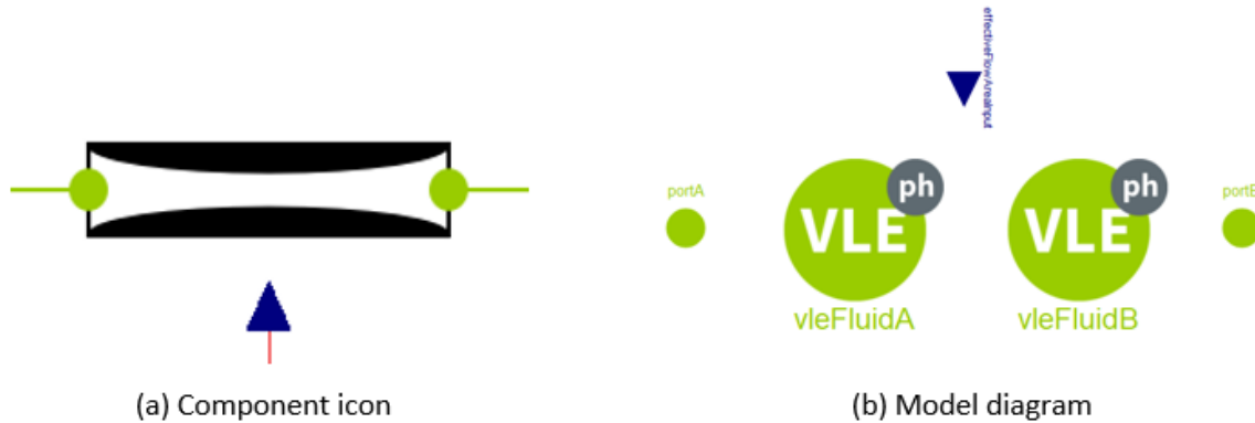
Figure 5.4 (a) shows the flow restrictor icon as it is represented in the complete model. (b) shows the model diagram of the flow restrictor including the elements the component is made of.
