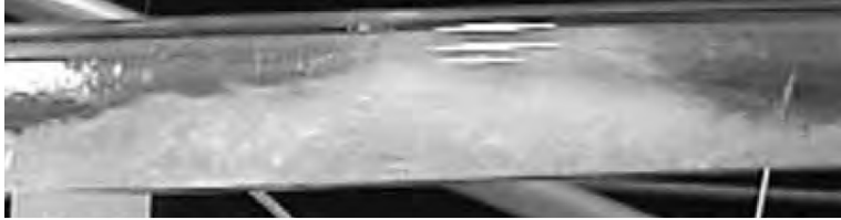
Figure 2.11: Roll wave observed in laboratory from previous experiments for air/water systems.
