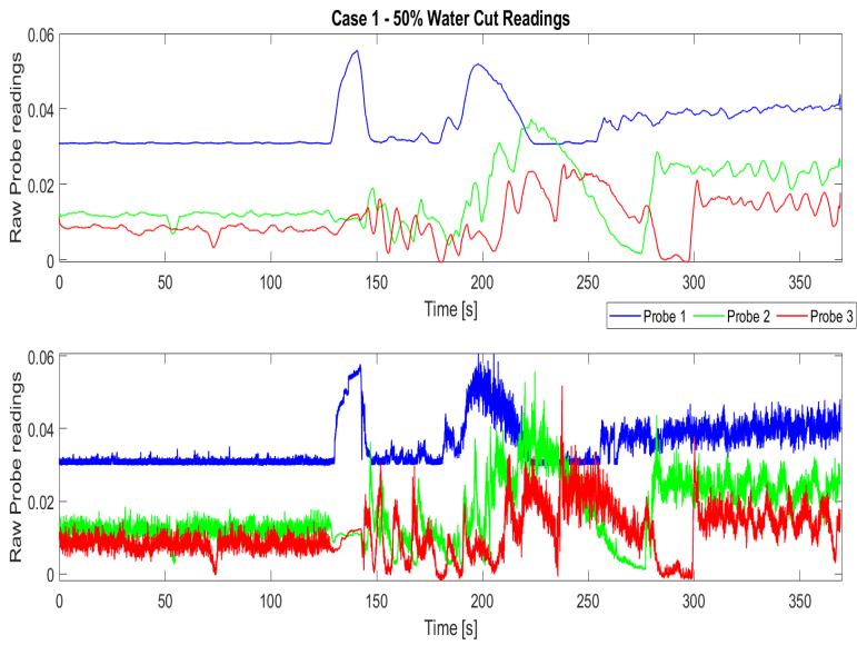
Figure 5.44: Plot showing experimental data for Case 1 with 50% water cut
