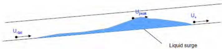
Figure 2.30: Layout showing characteristic phenomenon of surge wave formed by dip geometry.
