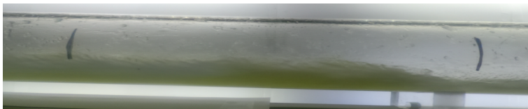
(b) Larger wave following the first wave, more messy and foamy at the top. Liquid distribution is unclear
