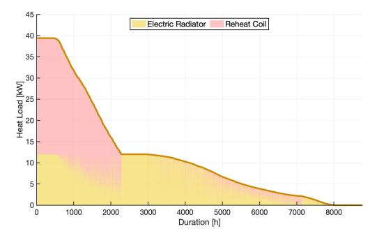
Figure 7.6: Base Case Heating Duration Curve
