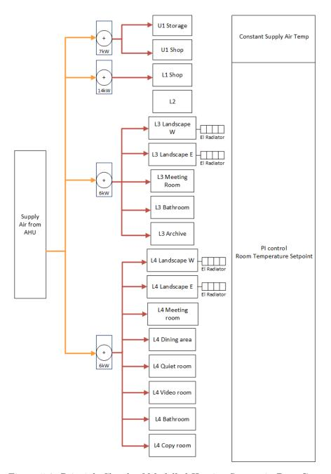
Figure 5.6: Principle Sketch of Modelled Heating System in Base Case
