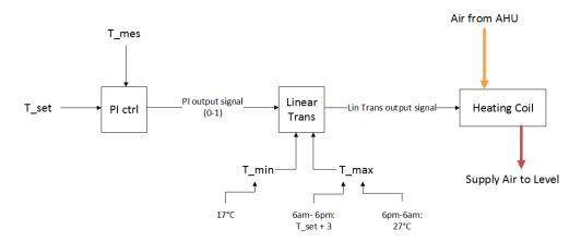
Figure 5.7: Reheat Coil Connection Diagram
