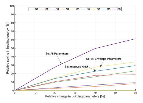
Figure 7.14: Comparison of Relative Heat Energy Saving of Rehab Scenarios
