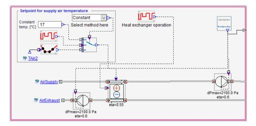
Figure 5.5: AHU Schematics in IDA ICE
