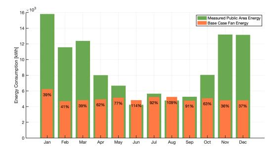
Figure 7.13: Public Area vs Simulated Fan Energy
