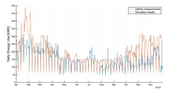
Figure 7.11: Arne Rønning Measured vs Simulated Daily Energy Use
