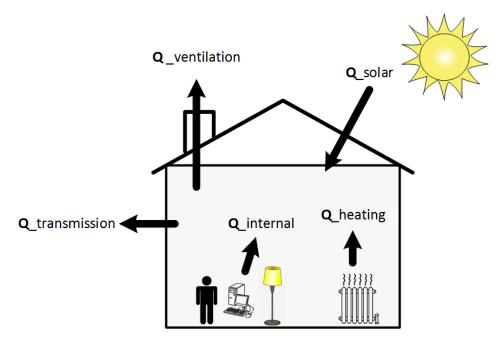
Figure 2.3: Principle Sketch of Heat Balance
