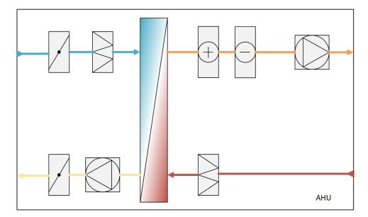
Figure 2.6: Principle Sketch of AHU
