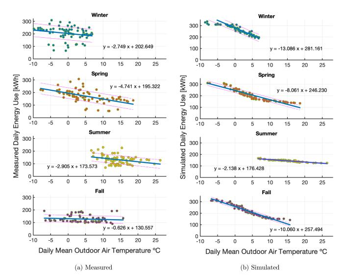
Figure 7.12: Arne Rønning Seasonal Analysis of Measured and Simulated Energy Use
