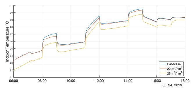
Figure 7.23: L4 Meeting Room Indoor Temperature With Improved Air Flow Rates
