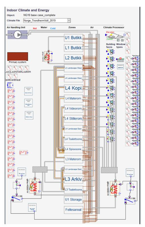
Figure C.1: Base Case Schematics Mode Interface
