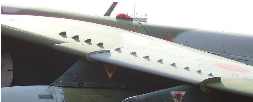
Figure 2.3: Vortex generators on an airplane wing [11]
