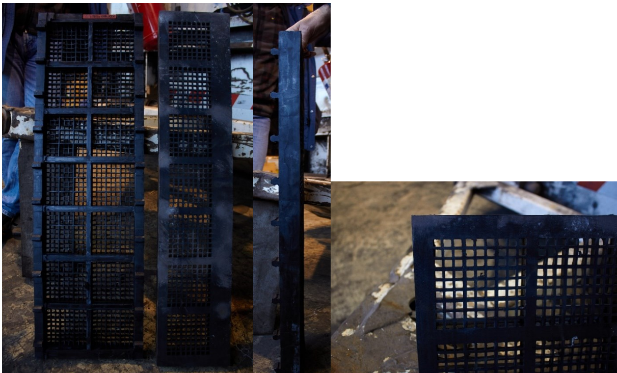
Figure 12 From left to right, detail of front and underside of the screen panels, side view of the screen panel and detail of the perforated net.
