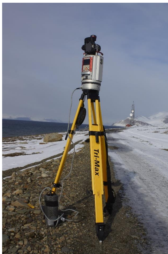
Figure 41 Laser scanner employed to obtain the DTM of the slope
